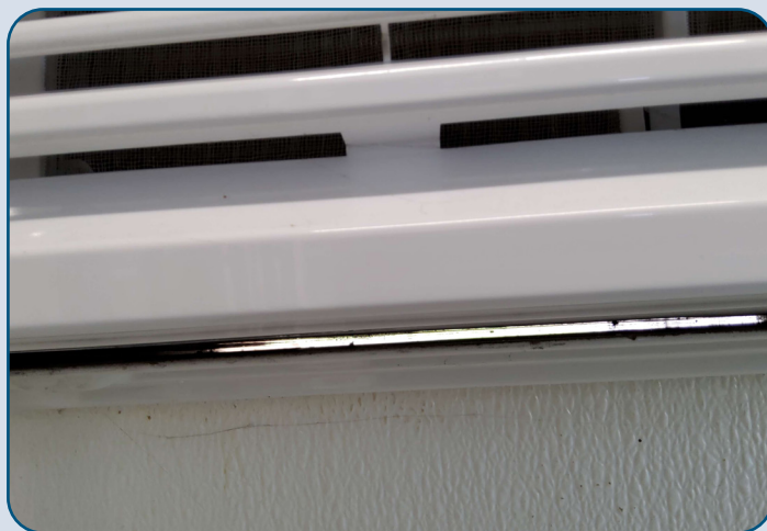
Figure 109: 360T MLG15 Failed Sealant.
