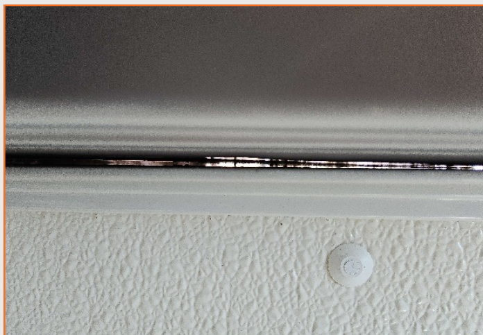
Figure 98: 360T MLG14 failed HVAC unit seal.
