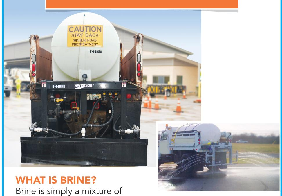
salt and water. We typically pre-treat our roads and bridges with it before a winter storm hits. It helps prevent ice or snow from sticking to the surface as precipitation starts. Winter precipitation can be very challenging to clear. Brine helps us in the early stages of a storm, before we begin other de-icing and plowing operations. Drivers should always slow down and pay close attention during storm conditions.
