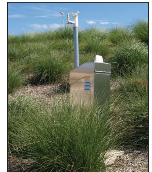
Field Controller / Wind Sensor on President George Bush Turnpike
